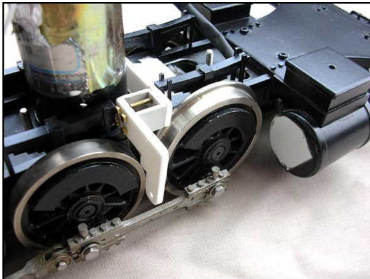
Figure 4: The above picture demonstrates the support bracket in position, prior to the 0.5mm styrene cover being applied over the packers, and the inside of the packers being filled with epoxy.
