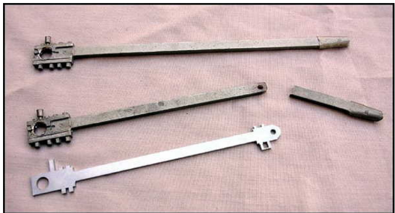
Figure 7: Use the laser cut main rod as a pattern to set out the hole to be drilled in the BBT main rod end.
