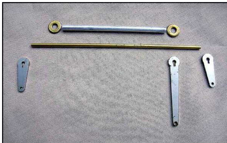
Figure 49: Bell rig extension parts.
