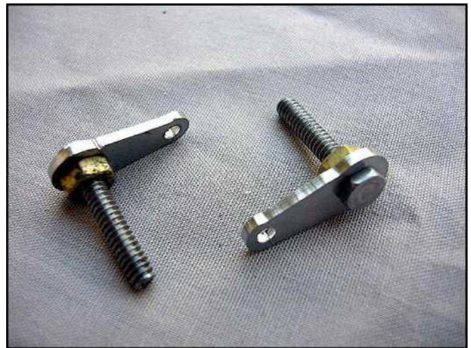
Figure 45: Two eccentric cranks ready for installation onto the 3rd Driver wheels.
