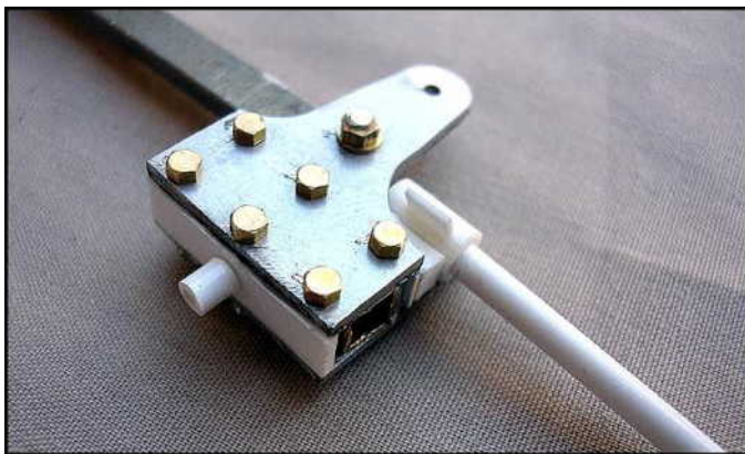
Figure 13: Note my oil cups are too tall, and were later shortened, as they bind with other parts of the valve gear!
