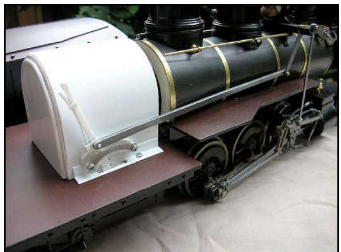
Figure 71: Now shown with the Johnson bar moved into the forward position:
