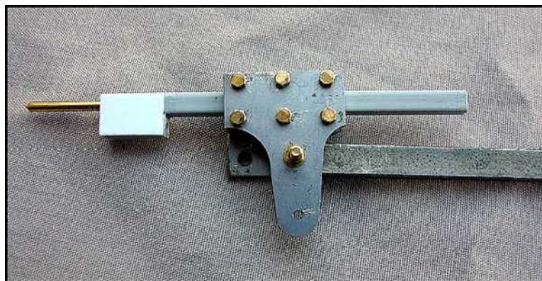
Figure 10: Note how the 6 bolts holding the crosshead together have a clean bolt head to the outside, while the main rod has the nut and washer exposed.
