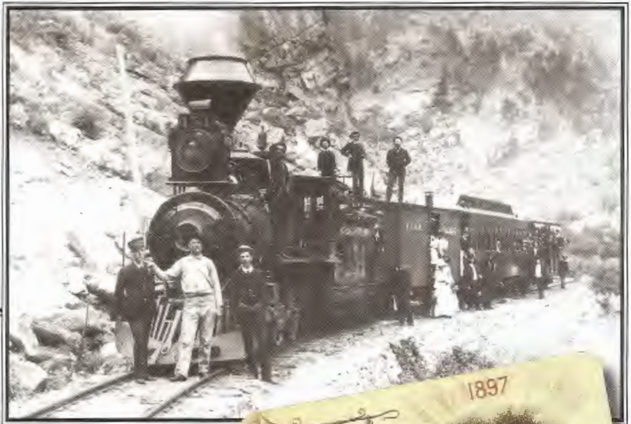
Right: CC #154, with an extended smokebox and diamond stack, heads a GSL&P train on the Horseshoe Curve in Boulder Canyon on August 1, 1886. Photo by Joe Sturtevant.
