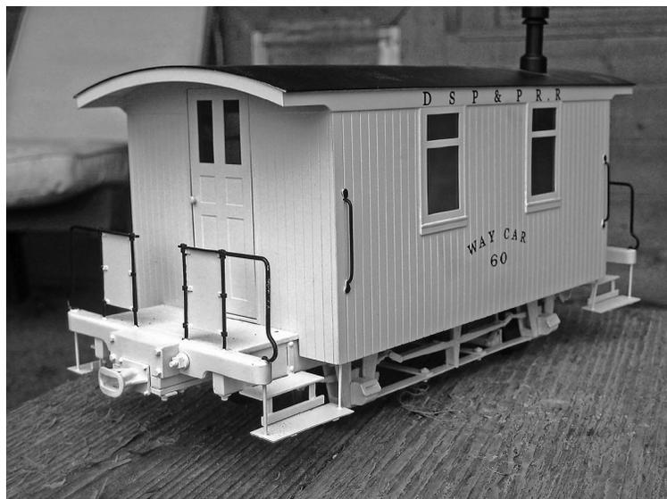
Builder's photo end view of Accucraft waycar showing solid panels in end rails and side window treatment.
