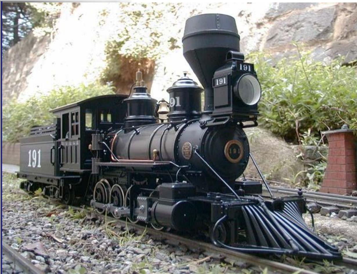
The model represents the #191 as it looked when rolled out of the shop with the new DSP&P numbering and UP colour scheme in 1885, within a year the DSP&P lettering on the cab was replaced by DL&G as the line again re-organised... the old west was so short lived.. I've been bashing locos for this era longer than the era actually lasted!
