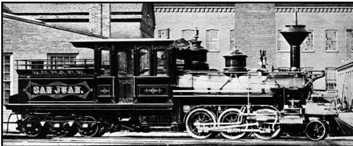
The '*San Juan*' of 1878 was the first full 2-6-6T delivered to the South Park, complete with pilot truck. The first South Park Mason, '*Oro City*' was delivered as a 0-6-6T, and later retrofitted with a pilot truck.
