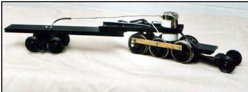
Barry also initially used a PVC pipe clip between the chassis and frame as a bearing pad, but we changed it as part of the spring rigging design in chapter 2. The tender deck assembly from chapter 2 also needs to be sandwiched between the two frame channels, with the deck flat down on top of the rear channel.
