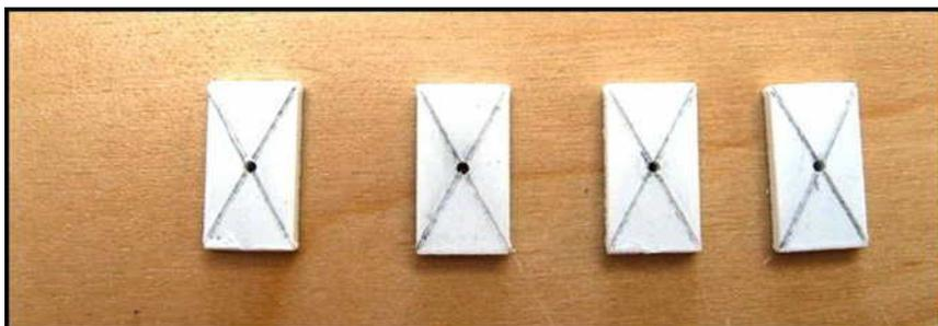
I'm lucky enough to own an electric sander. This turned out to be a tremendous time saver. It allowed me to accurately bevel the edges of the plates with relative ease. I used double-sided tape to temporarily attach the plates to the top of a stick. This provided a stable platform to perform the sanding. I have to admit that determining the angle of the sander was a bit trial and error but, by taking a little off at a time, I got the hang of it pretty quickly.
