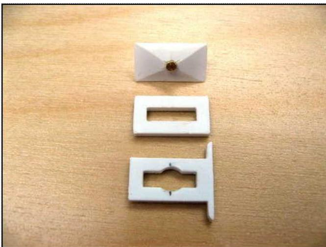
The parts for the truck beam caps are shown below. The top piece is the end plate after beveling. As will be mentioned later, I permanently glued one side frame to the truck beams. I found it desirable to make the other side frame removable just in case the wheel sets needed to be replaced in the future. For the side frame that is glued to the beams, the 3 parts are glued together and then glued to the side frame.
