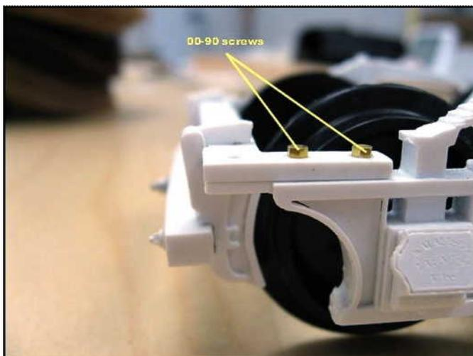
The brake assemblies were attached using #00-90 hex head bolts. I drilled the holes in the brake hanger beam then aligned and marked for the holes in the top of the side frame. I used a #56 drill for the #00-90 bolt holes in the hanger beam and drill size #58 for the tap size in the side frame. Here's a close up below.
