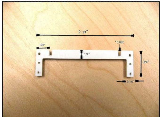
I reinforced the beam, on the underside, with a piece of 0.060" x 0.125" styrene. The reinforcing piece is cut to fit between the insides of the side frame extensions. The combination of the two thicknesses was just right to allow the brake shoes to slide onto the assembly.
