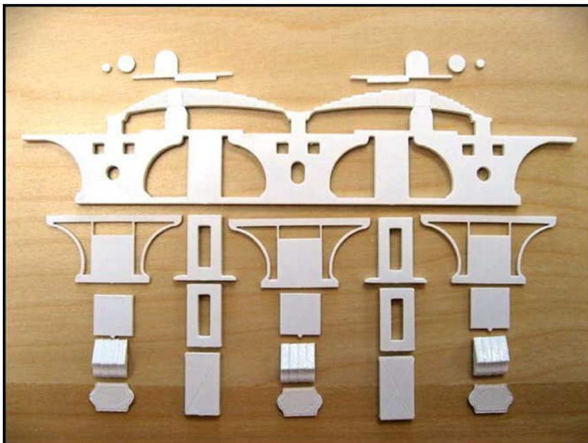
The photo below shows the parts for the truck beams and pivot plate.
