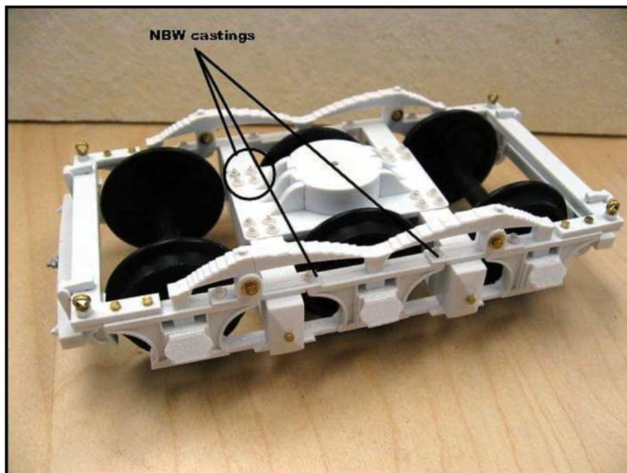
The other parts I added are the eyelets for the safety chains. I found the brass eyelets at Michaels craft store. They actually look more like small cotter pins. They are shown in the insert in the next photo. I made mounts for the eyelets by taking 1/8" dia. styrene tubing, filing the tops of each with a round file, and cutting them to length. I then glued the eyelets into the tubing using thick CA.
