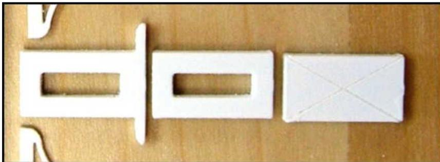
One of the most difficult parts of this kit, I think, is the beveling of the truck beam end plates. The first thing I did was to drill holes in the centers of the plates for 00-90 screws. You need to do this first to ensure they are centered.
