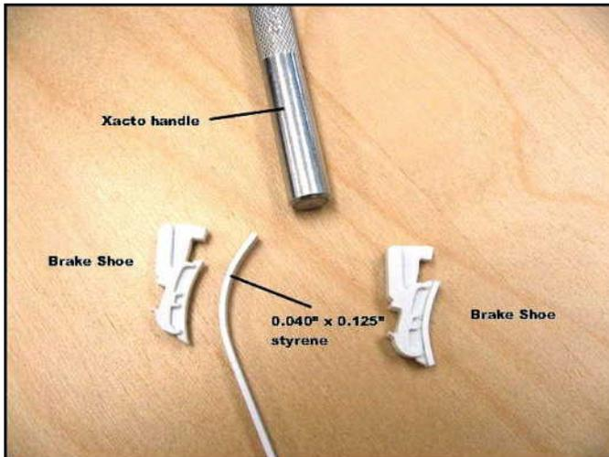
The assembly steps were as follows: attach brake shoes to upper hanger beams; attach lower beam to brake shoes; and measure and drill for screws that will hold entire assembly to truck.
