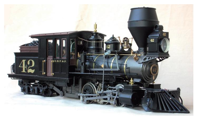
The chassis was a custom designed effort via 'Barrys Big Trains' in Arizona, and features cast magnesium main rod and side rods, cast from CNC machined masters developed in 3D cad, and finally a laser cut stainless steel valve gear set, cut here in Melbourne.
